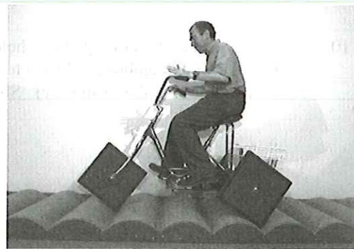
The picture above shows Stan Wagon riding his special square-wheeled tricycle. This tricycle is on display at Macalester College in St. Paul, Minnesota. Reprinted with permission.
